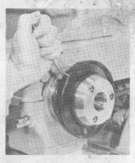
STEP 1 With lathe in back gears, mount chuck on threaded spindle using a piece of %" drill rod in spanner hole to spin chuck securely on to spindle.
