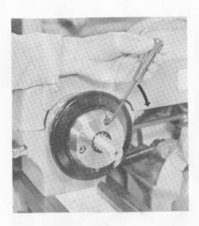
STEP 5 Insert hex-key into any one of three pinions and turn to tighten the chuck securely.
