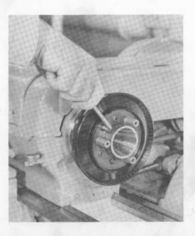
**STEP 4** Remove three of the six body retaining screws (remove every other screw.) Break loose three remaining body retaining screws and retighten lightly to permit radial adjustment.
