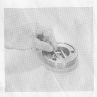
STEP 1 Place the spacer bars on the collet bearing surface of the nose.
