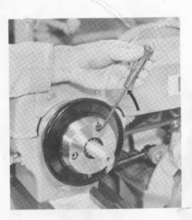
STEP 6 To loosen chuck insert hex-key into any one of the three pinions and turn.
