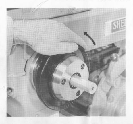
STEP 7 Turn handwheel to open collet.
