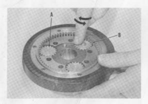
**STEP 4** Assemble the handwheel by engaging its ring gear with one pinion gear (see "A" above).
