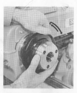
**STEP 3** To prevent crossed threads on pinions turn handwheel one quarter turn in opening direction and then in closing direction until nose starts to close collet.
