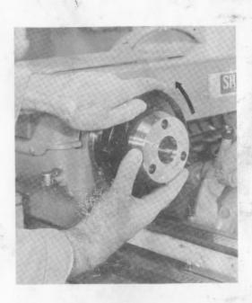
STEP 1 Turn handwheel to remove the nose.
