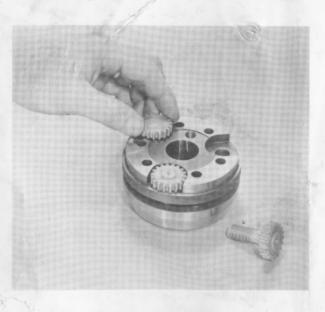
STEP 3 Screw the three pinions into the nose through the holes in the body until they are finger tight. Note that pinion threads are LEFT HAND.
